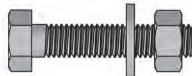
(4) M8 x 40mm HEX BOLT (2 Washers, 1 Lock-Nut)
