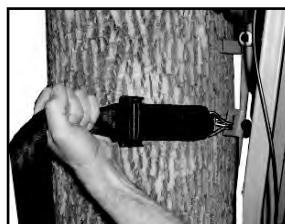
FIGURE 3: SECURE YOUR HARNES, PULL EXCESS STRAP TO TIGHTEN AND SECURE STAND TO TREE
